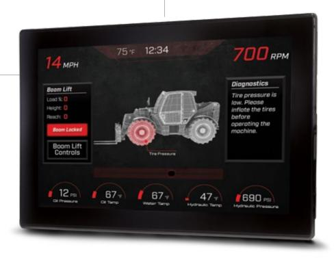
Murphy brings a whole new experience to your applications with the PowerView 1100. This large 10.6-inch display features a high-speed processor that allows you to bring even more into your application. In addition to providing vital engine information, the PV1100 packs an infotainment hub in the cab with media playback from your phone via USB. It also boasts AM/FM stereo, Bluetooth and Wi-Fi connectivity.
