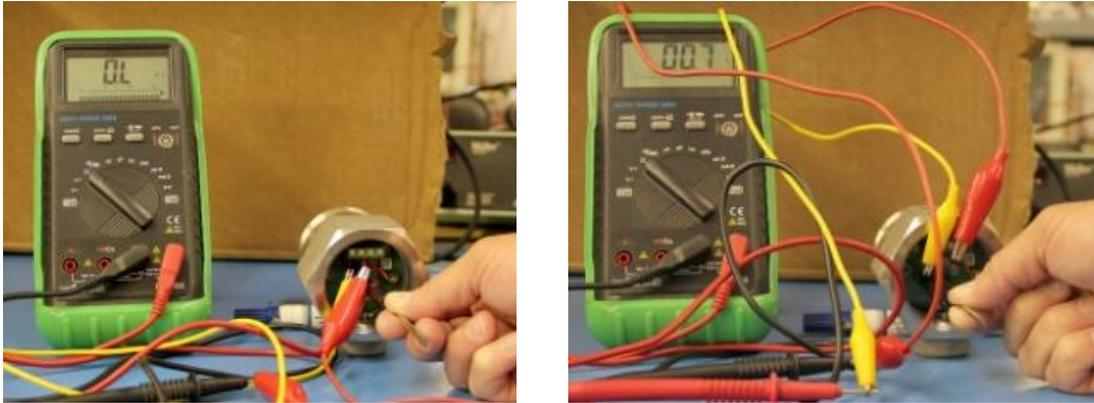
1. Figure #1 Switch operates normally
