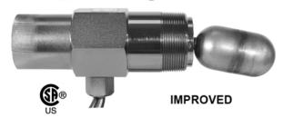
**LS200** Liquid Level Switches with 2" NPT mounting are float activated to operate an electrical SPDT snap switch (optional DPDT on some models) for alarm or shutdown of an engine or electric motor. The LS200 connects directly into the vessel wall and can be used with a Murphy weld collar (P/N 15050375) or Murphy external float chamber (P/N 15700799). L1100 models (1-1/2" NPT) are also available.
