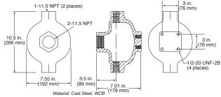
Operating Pressure: 2000 psi (13.8 MPa) [138 bar] Operating Temperature: 400 deg F (204 deg C)
