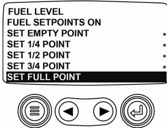
The following screen is displayed and now the resistive value that represents the Full point from the non-Murphy fuel sender must be sent to the PV101. While sending the resistive value, select **[YES]** and the PV101 will have a new Full fuel setpoint setting.
