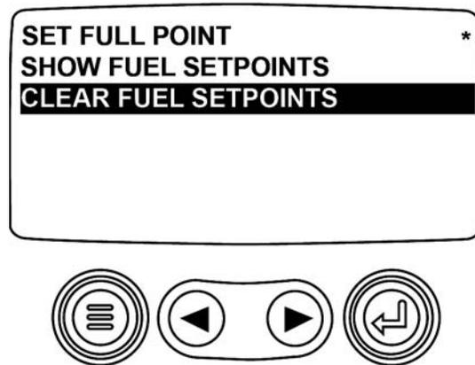
**NOTE:** The SET EMPTY POINT, SET 1/4 POINT, SET 1/2 POINT, SET 3/4 POINT and SET FULL POINT must be programmed before continuing.
