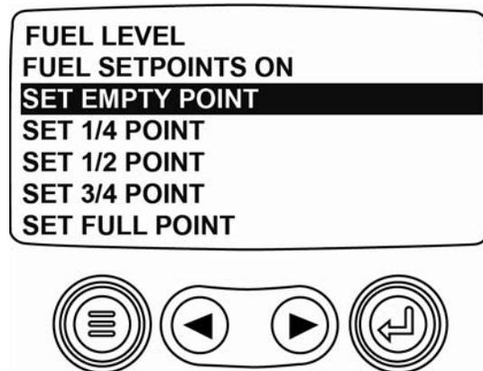
**NOTE:** The fuel tank must be empty to begin this process.
