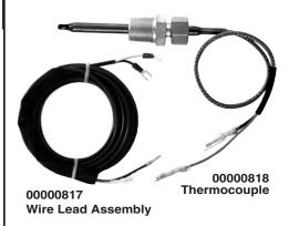
**Thermocouples** 00000818 and 00003488 can mount in the engine manifold or in 2 to 3-1/2 in. (51 to 89 mm) diameter exhaust ports. In turbo-charged engines, a thermocouple mounts between the engine and the turbo. Thermocouple 00000818 is a grounded, type K (Chromel Alumel). Thermocouple 00003488 is ungrounded type K (Chromel Alumel).
