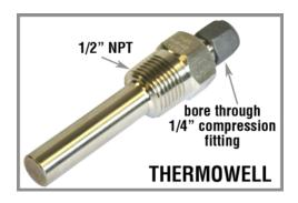
Thermowells are available in 2", 4-1/2", or 7-1/2" lengths for insertion depth and have a  $\frac{1}{2}$ " NPT process connection. They are supplied with a standard stainless steel compression fitting for securing the thermocouple in the thermocouple at the appropriate depth. In low pressure applications the thermocouple can be inserted directly into the process through a standard  $\frac{1}{4}$ " SS tubing compression fitting.
