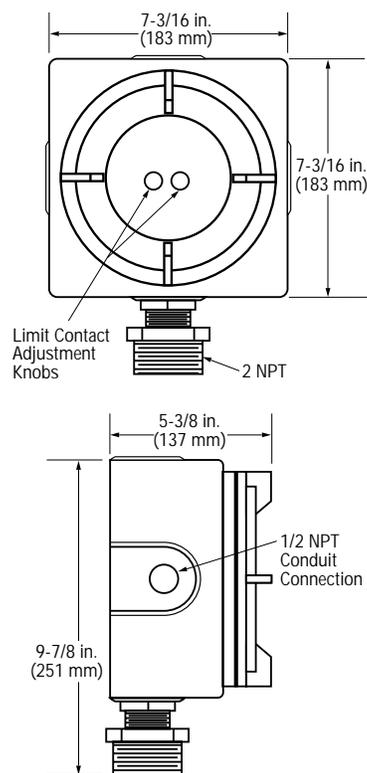
\* The PT167EX is CSA listed for ranges 100 to 5000 psi (689 kPa to 34.5 MPa) [6.89 to 344.74 bar].
