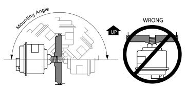
**3.** Locate the unit in place and secure it by tightening the 1/8-27 NPT fitting into the desired location (do not overtighten). **DO NOT TWIST CASE.**
