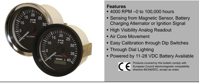
The AT Series tachometers are rugged, transistorized instruments with solid-state circuitry for indication of engine RPM. They are equipped with a bracket for mounting into a standard 3- 3/8 in. (86 mm) dash mounting hole. A full 270° sweep of the pointer gives an accurate indication on a large easy–to–read scale and the dial can be illuminated for night reading. The ATH Series models are also equipped with hourmeter to record the elapsed running time of an engine.
