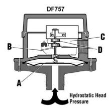
As the liquid level rises, hydrostatic head pressure is applied to the diaphragm **A**. The diaphragm is forced upward forcing the actuator arm **B** to activate the snap-switch **C**.
