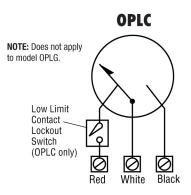
Contact Rating: 1 SPDT; Center off; 2 A, 30 VDC, 0.1 A, 125 VAC pilot duty
