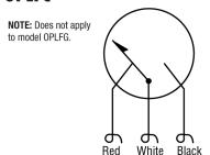
Contact Rating: 1 SPDT; Center off; 2 A, 30 VDC, 0.1 A, 125 VAC pilot duty
